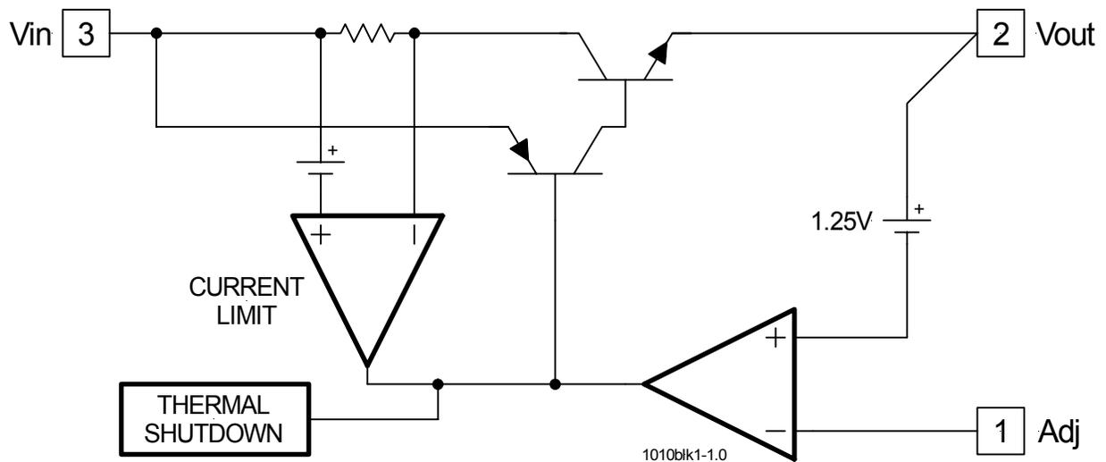
Figure 2 - Simplified block diagram of the IRU1010
