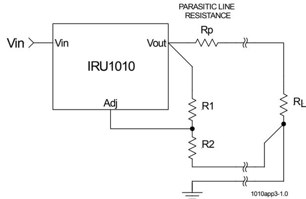
Figure 4 - Schematic showing connection for best load regulation
